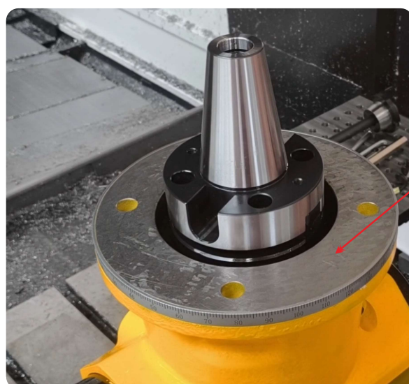
16. 清洁侧铣头表面 Clean the surface of the side milling head
